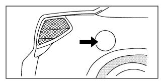
To open the fuel door, apply pressure in the center of the rear edge of the fuel door and it will pop open.
